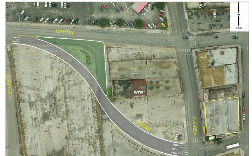
Realignment of Pecan Street at Martin Street
