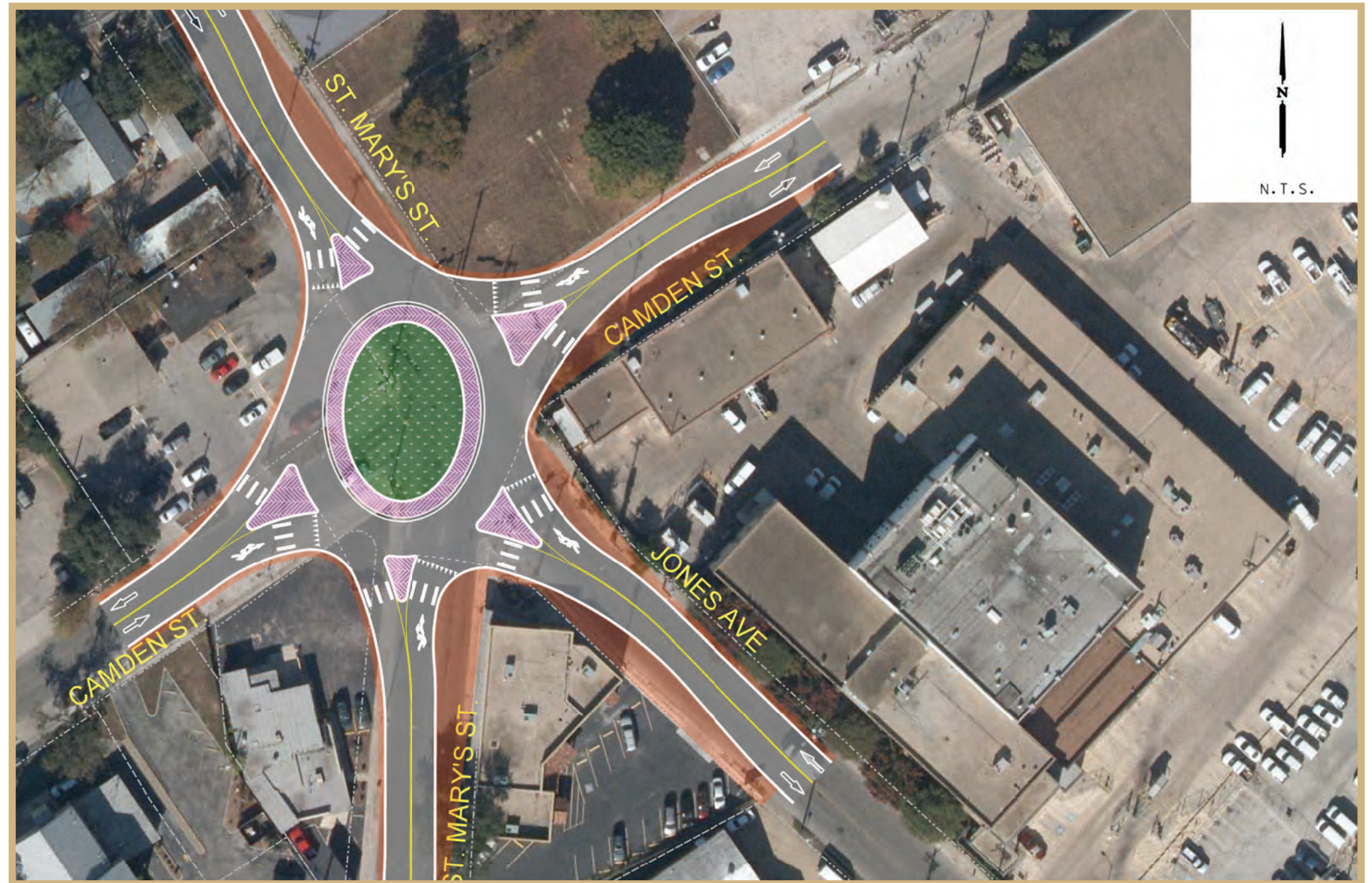
Figure 3-68: Roundabout Concept for Intersection of Jones, Camden and St. Mary's
