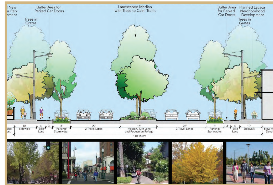
Proposed Section and Examples: four-lane divided roadway with bike lanes.
