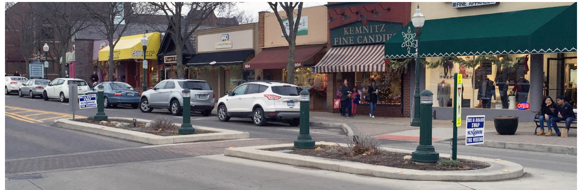
Midblock Crossing With Landscaped Refuge Island, Plymouth, Michigan
